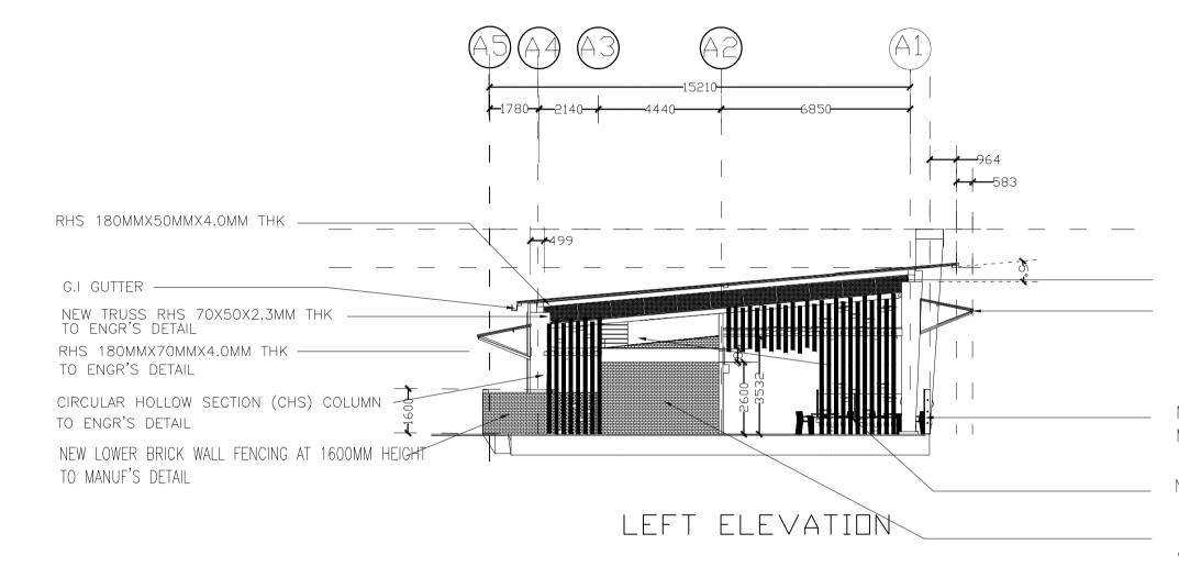
1298mm x 600mm STAINLESS STEEL WIREMESH NETTING 2MESH WITH PANEL, WIRE 0.55MM, HOLE 2MM NEW POLYCARBONE ROOFING WITH STEEL SUPPORT BELOW TO DETAIL
